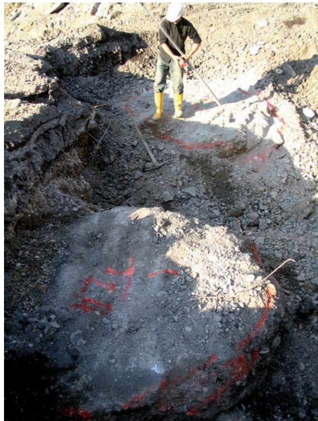
Fig. 1: Excavated test columns Image: PORR
