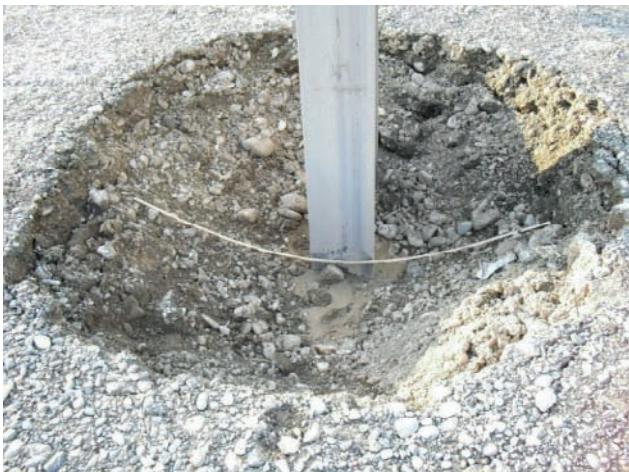
Crater after trial pile drive Image: PORR
