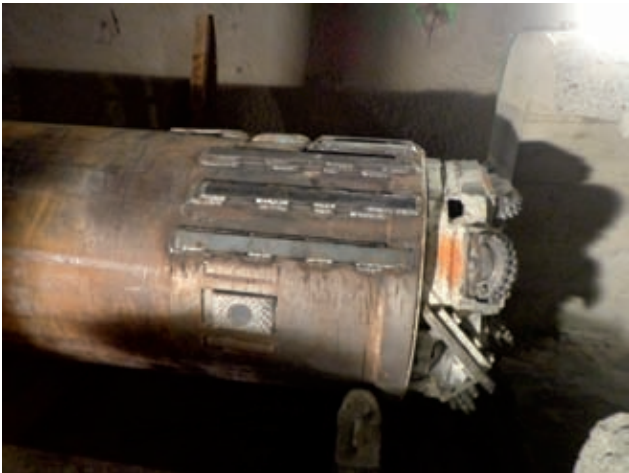
Cutter head of the 800 mm large-hole drilling Image: PORR
