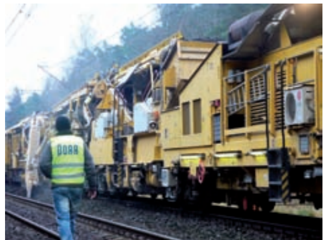
Use of the RM 801-2 bedding cleaning machine on Line 273 Image: PORR
