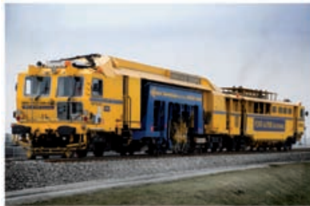
Line 132, UNIMAT 09-32/4S Dynamic tamping machine of Austriarail Image: PORR
