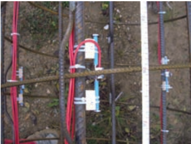
Instrumentation of static test pile Image: PORR
