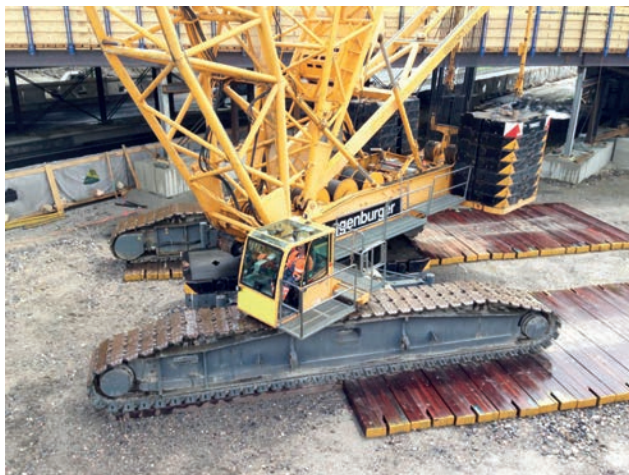
Installation of 750t crawler crane Image: PORR AG
