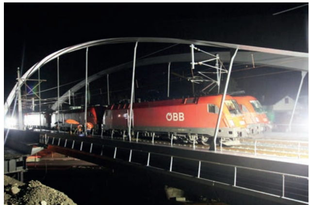
Load test using 6 "Taurus" locomotives weighing 86t each Image: PORR AG
