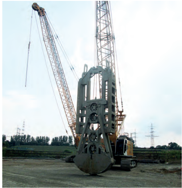
Diaphragm wall grabber Image: PORR AG
