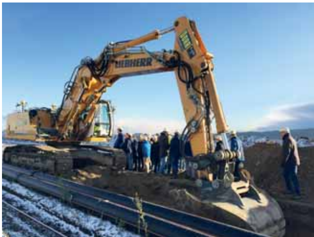
Krems School of Technology field trip with the advance excavator with its trapezoidal bucket and 3D steering Image: PORR AG
