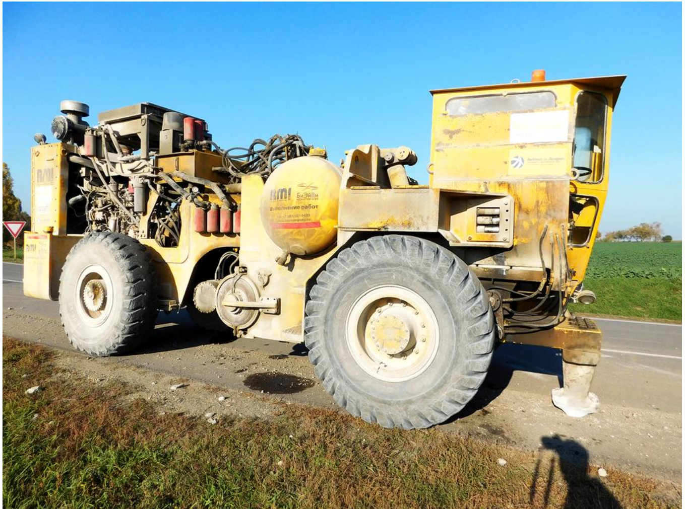
RB 500 resonance breaker – construction machine for demolishing the concrete substructure. Image: PORR AG
