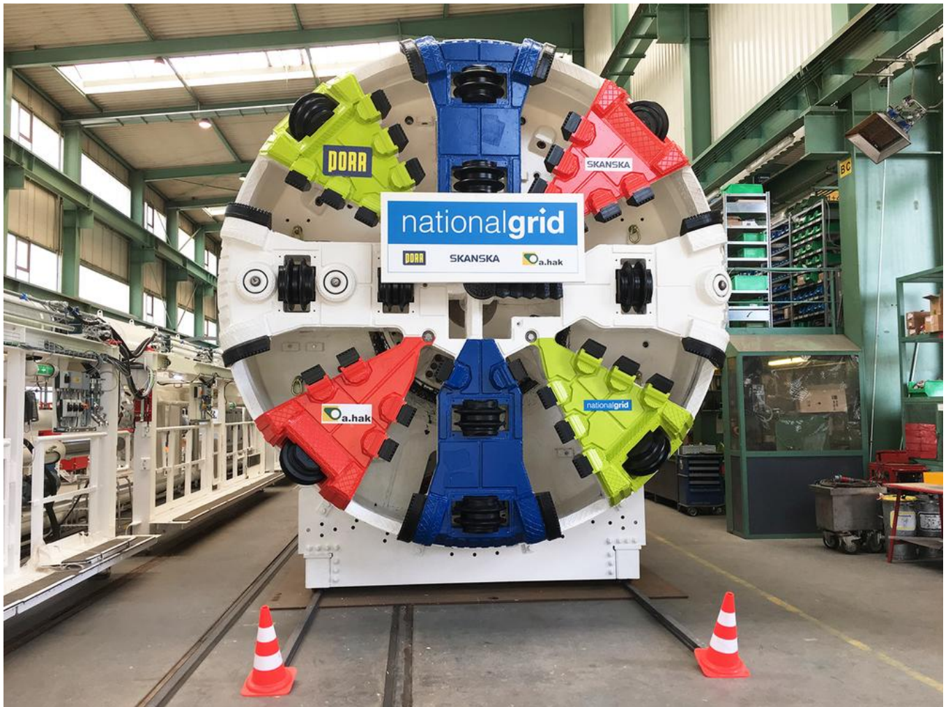
The tunnel boring machine used to excavate the tunnel underneath the River Humber. Image: Herrenknecht AG
