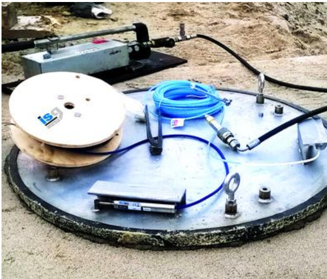
Foot pressure gauge pad before being installed on the reinforcement cage. Image: isg
