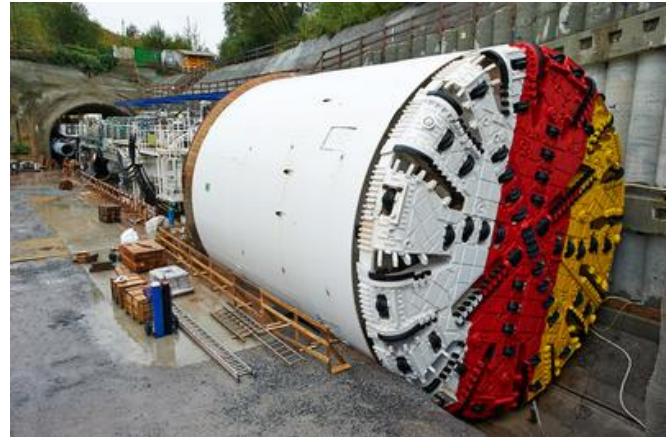
The “KORA” TBM was assembled in the Mitterpichling construction pit. The drill bears the Carinthian state colours. Source: Toni Rappersberger
