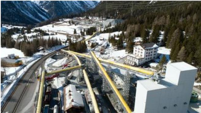
The consortium operates a gravel plant in Preda, which can process up to 4,000t of excavated material each week. Source: Torsten Schaarschmidt, Pöyry Schweiz AG
