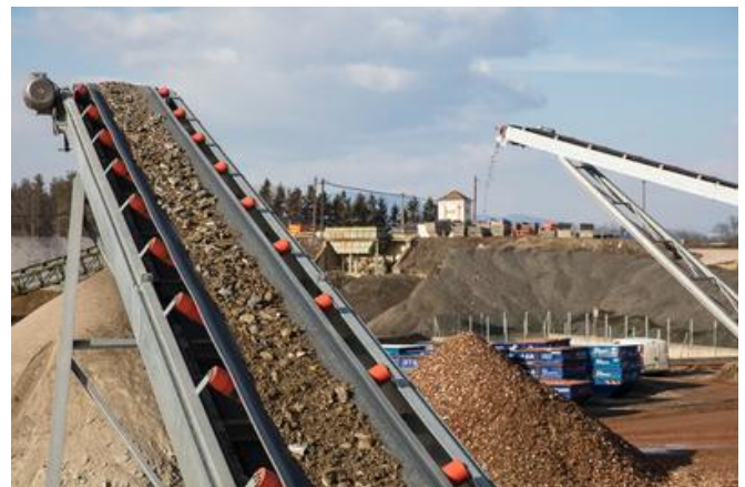
Conveyor belts with medium fraction and the end product. Source: Daniel Ulbricht-Sundt
