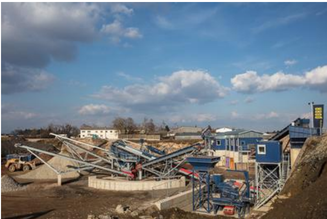
The light material separator with dewatering screen in the first extension. Source: Daniel Ulbricht-Sundt
