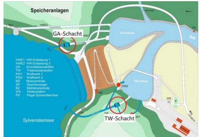
Overview plan of the Sylvenstein Reservoir, showing the sluice tunnel in the north and the headrace tunnel in the south. Source: Wasserwirtschaftsamt Weilheim
