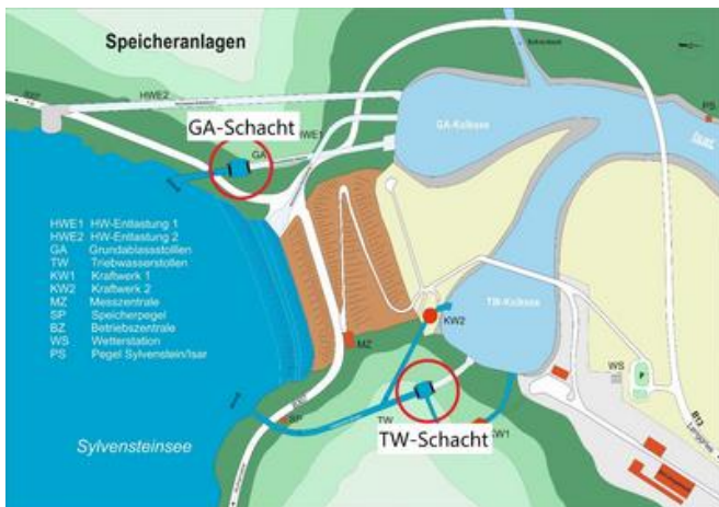
Overview plan of the Sylvenstein Reservoir, showing the sluice tunnel in the north and the headrace tunnel in the south. Source: Wasserwirtschaftsamt Weilheim
